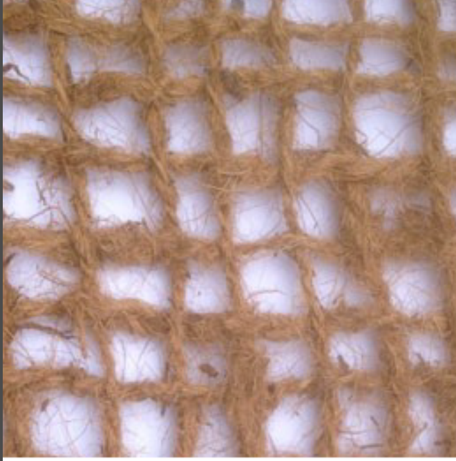
Coir stabilising netting for the front bank before planting
